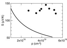
**Fig. 3.** Pisarenko relation of Seebeck coefficient at 300 K versus hole concentration for PbTe (solid line) compared to the results measured on every Tl-PbTe sample prepared for this study.
